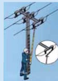
Operating disconnect switches
